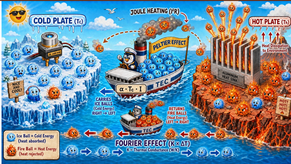
Figure 1: The TEC island analogy. The Peltier ferry carries heat packets from the cold island to the hot island, while the electrical input adds Joule heat that must also be rejected on the hot side. The ferry’s smokestack represents total Joule heating Q_{\text{Joule}} = I^2R . In the water, Fourier conduction Q_{\text{Fourier}} = K \cdot \Delta T continuously leaks heat from the hot side back to the cold side, opposing the Peltier pumping.
