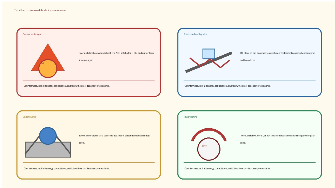
Figure 3. Four villains in the thermistor failure zoo: overcurrent, board bending, solder stress, and rework overheating.
