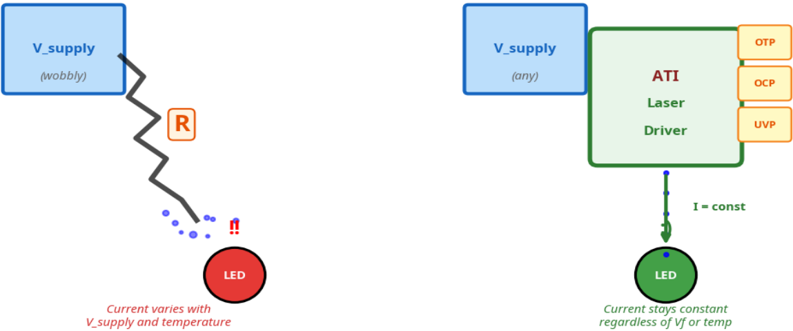
Figure 2: A ballast resistor (left) provides no regulation—current fluctuates with every supply voltage change. A constant-current driver (right) maintains precise, stable current regardless of input variations, with built-in OTP, OCP, and UVP protection.
