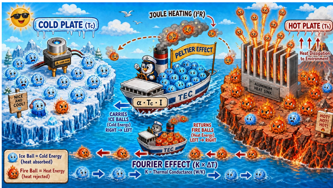
Figure 1: The TEC island analogy. The Peltier ferry carries heat packets from the cold island to the hot island, while the electrical input adds Joule heat that must also be rejected on the hot side. The ferry's smokestack represents total Joule heating Q_{\text{Joule}} =
