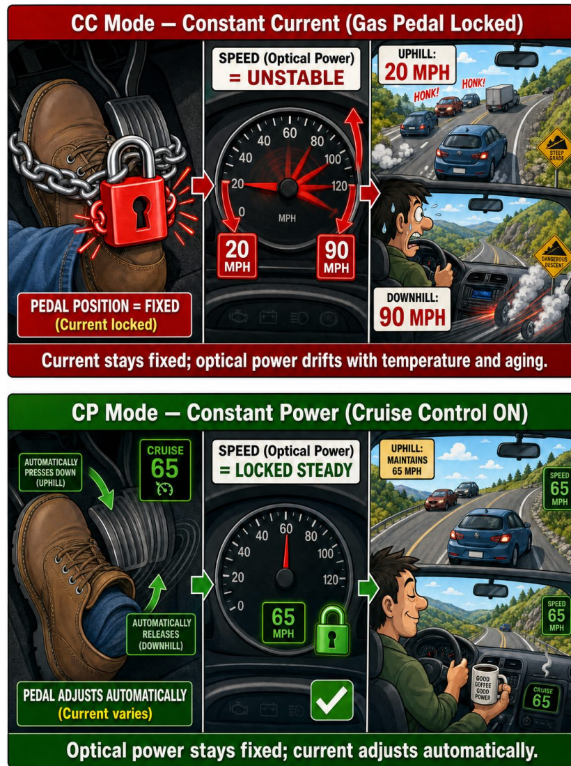
Figure 4. CC mode is like locking the gas pedal at one position — the car's speed (optical power) varies as the road changes (temperature, aging). Going uphill the car slows to 20 MPH; downhill it rockets to 90 MPH. CP mode is like cruise control — the speed is locked at 65 MPH and the gas pedal moves automatically to maintain it regardless of road conditions. Design rule: in CP mode the current can climb to hold power as the diode ages or heats, so a current limit must stay active underneath the optical loop.
