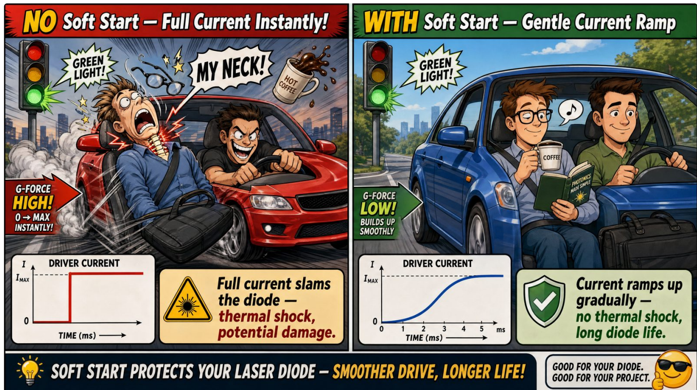
Figure 6. Soft start is like accelerating a car from a stop. Without soft start (left): the driver floors the gas pedal at the green light — passengers' heads snap backward into the headrest, coffee flies everywhere, neck whiplash. The current waveform shows an instant spike. With soft start (right): the driver eases onto the gas gently — passengers sip coffee peacefully, heads stay upright, smooth comfortable ride. The current waveform shows a controlled ramp. Design rule: treat turn-on behavior as a protection feature, not a convenience. Soft start protects your laser diode — smoother drive, longer life.
