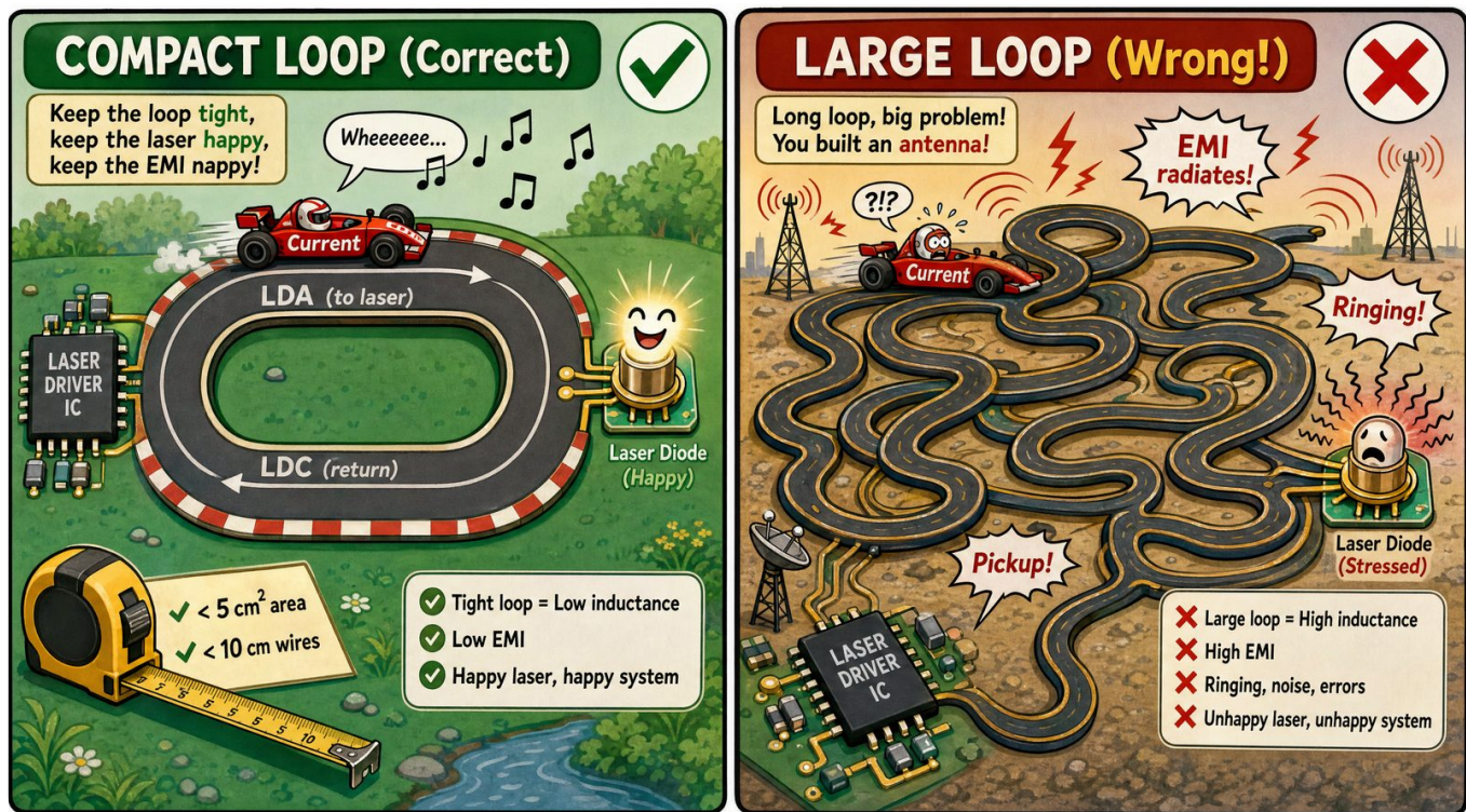
Figure 8. Output-loop layout: a short, tidy racetrack (loop area <math>< 5 \text{ cm}^2</math>, wires <math>< 10 \text{ cm}</math>) stays quiet, while a long wandering loop becomes an antenna for ringing and EMI. Design rule: route the outgoing (LDA) and return (LDC) conductors together to minimize enclosed area.
