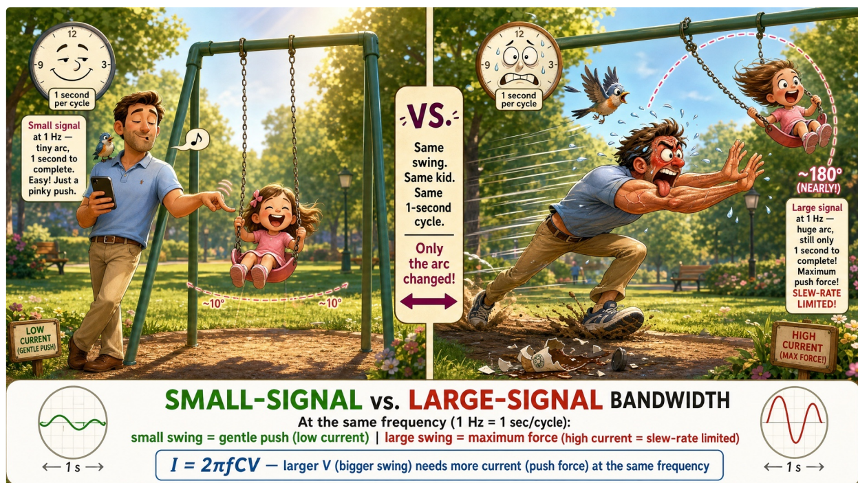
Figure 4 — The Playground Swing Analogy. Same swing, same child, same 1-second cycle (1 Hz). A small arc (small-signal) is easy — barely any push force needed. A huge arc (large-signal) that must complete within the same 1-second period requires massive push force (current). If the required force exceeds the pusher’s maximum strength (amplifier’s
