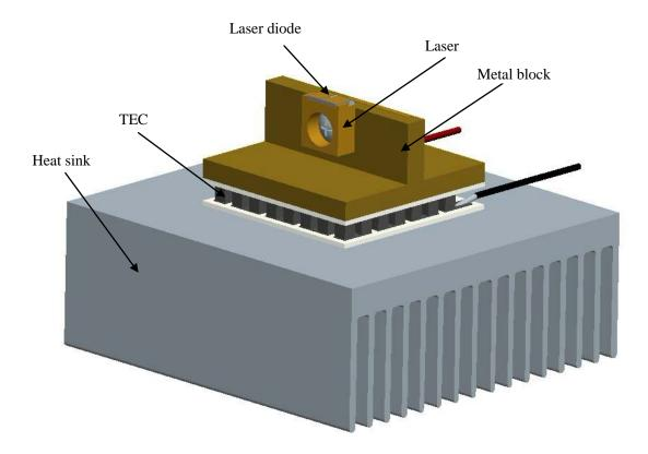
Note: Thermal conductive epoxy needs to be put between every two contact surfaces in this system.
