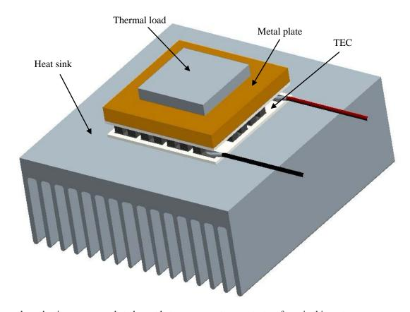
Note: Thermal conductive epoxy needs to be put between every two contact surfaces in this system.
