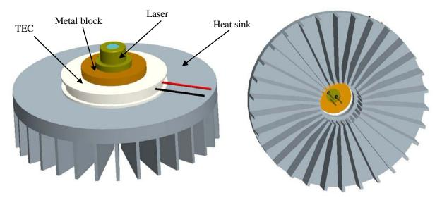
Note: Thermal conductive epoxy needs to be put between every two contact surfaces in this system.
