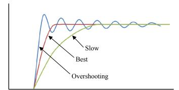
Figure 8. Rise Waveforms of VTEC
