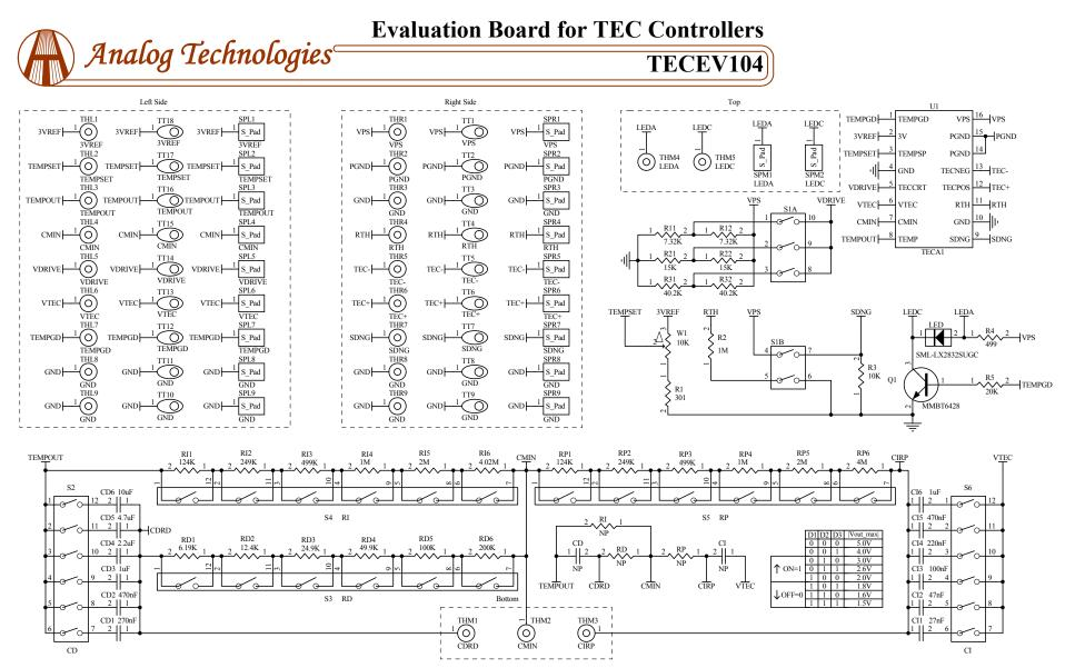
Figure 7. Schematic of TEC Controller Evaluation Board TECEV104
