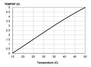
Figure 5. TEMPSP vs. Temperature
