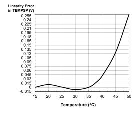
Figure 9. Linearity error in TEMPSP vs. Temperature
