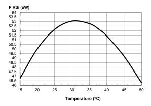
Figure 8. P<sub>Rth</sub> vs. Temperature
