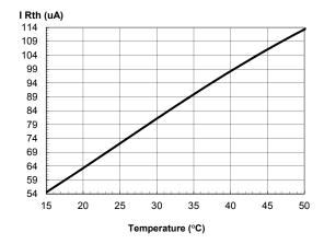
Figure 6. I<sub>Rth</sub> vs. Temperature
