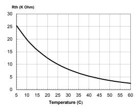
Figure 4. Rth vs. Temperature
