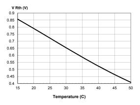
Figure 7.  $V_{Rth}$  vs. Temperature
