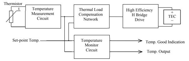
Figure 3. TEC Controller Block Diagram
