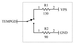
Figure 5. Internal Equivalent Circuit on TEMPGD Pin
