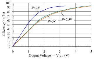
Figure 24. Efficiency vs. V<sub>OUT</sub>
