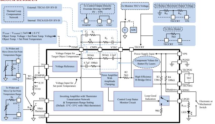
Figure 4. TEC Controller Functional Block Diagram
