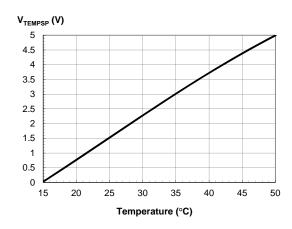
Figure 20. V<sub>TEMPSP</sub> (0V-5V) vs. Temperature
