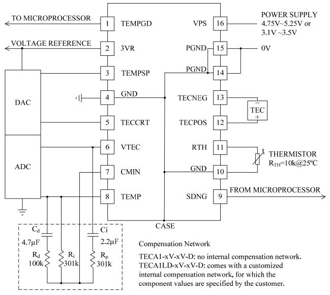
Figure 10. Microprocessor Based Application Circuit
