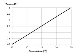
Figure 21. V<sub>TEMPSP</sub> (0.1V-3V) vs. Temperature
