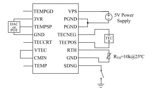
Figure 15. Control the Current Direction of the TEC Module by Pin 3 TEMPSP
