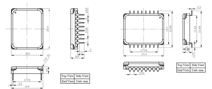
Figure 27.Dimensions of the SMT Package Controller of TECA1-XV-XV-S
