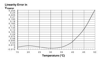
Figure 22. Linearity Error in  $V_{\text{TEMPSP}}$  vs. Temperature
