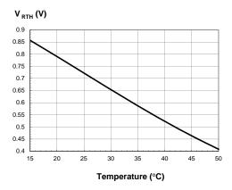
Figure 17. V<sub>Rth</sub> vs. Temperature
