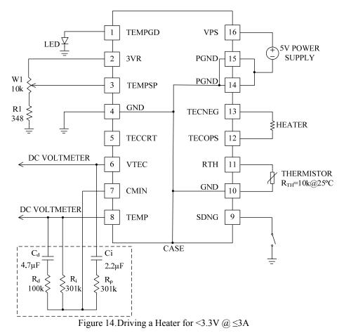
If  $V_{HTMAX}$ <3.3V, the part # is TECA1-5V-[ $V_{HTMAX}$ ]V-D. For example,  $V_{HTMAX}$ =2.5V, the part number will become: TECA1-5V-2.5V-D, when using a 5V power supply. If powered by a 3.3V power supply, the part number will be: TECA1-3V-2.5V-D.
