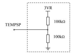
Figure 6. Internal Equivalent Circuit on TEMPSP Pin
