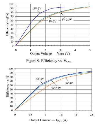
Figure 10. Efficiency vs. IOUT
