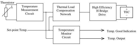
Figure 3. TEC Controller Block Diagram
