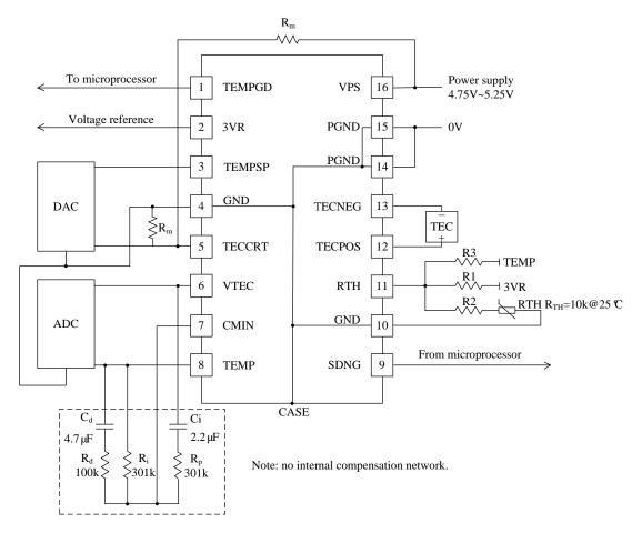
Figure 4. Microprocessor Based Application Circuit
