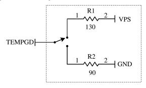
Figure 11. Internal Equivalent Circuit on TEMPGD Pin
