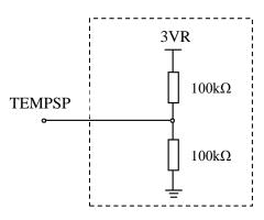
Figure 12. Internal Equivalent Circuit on TEMPSP Pin
