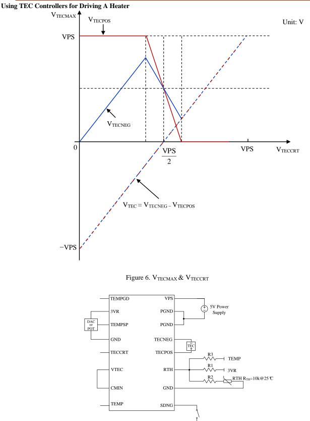
Figure 7. Control the Current Direction of the TEC Module by Pin 3 TEMPSP
