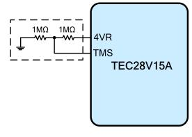
Figure 3. TMS Input Equivalent Circuit
