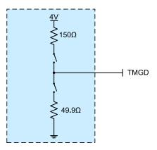
Figure 19. Output Equivalent Circuit for TMGD Pin
