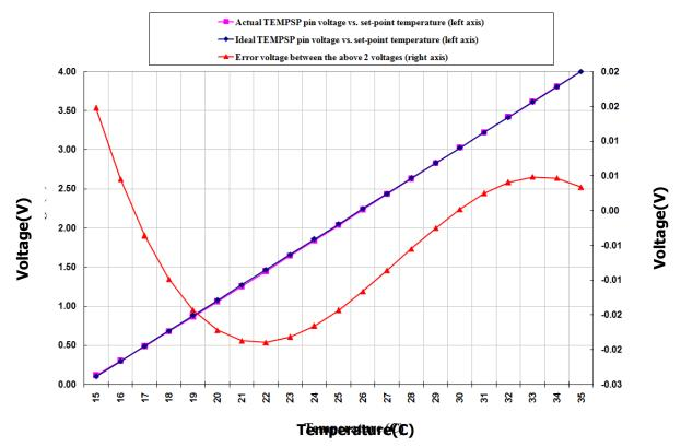
Figure 25. TMO Pin Voltage vs. Set-point Temperature
