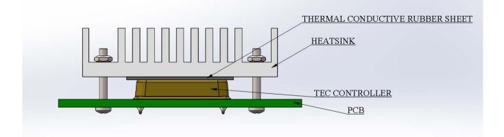
Figure 27. Transferring Heat with Heat Sink
