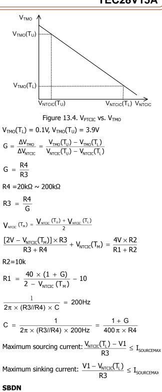
SBDN is suggested to be pulled up to VPS with a  $10\mu$ A current and contains a 1.50V logic threshold. Drive this pin to a logic-high to enable the TEC28V15A. Drive to a logic-low to disable the TEC controller and enter micro-power shutdown mode.
