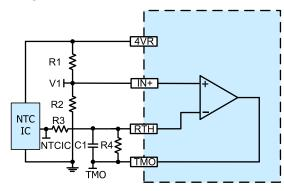
Figure 13.1. NTC IC temperature sensor
