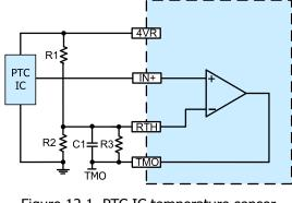
Figure 12.1. PTC IC temperature sensor
