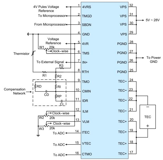
Figure 8.1. TEC Controller Connection
