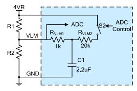
Figure 18. VLM vs. Cooling and Heating Control
