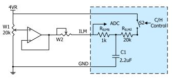
Figure 20. ILM vs. Cooling and Heating Control
