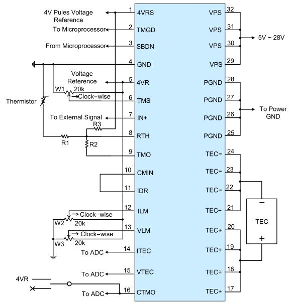
Figure 8.2. Connection for TEC28V15ADAPID & TEC28V15ASAPID
