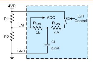
Figure 16. ILM vs. Cooling and Heating Control The switch S1 is closed @ heating, and open @ cooling
