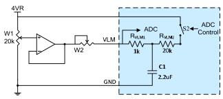
Figure 4. VLM Input Equivalent Circuit The switch S2 is closed @ heating, and open @ cooling
