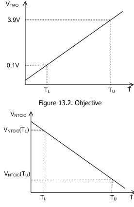
Figure13.3. Temperature vs. V<sub>NTCIC</sub>
