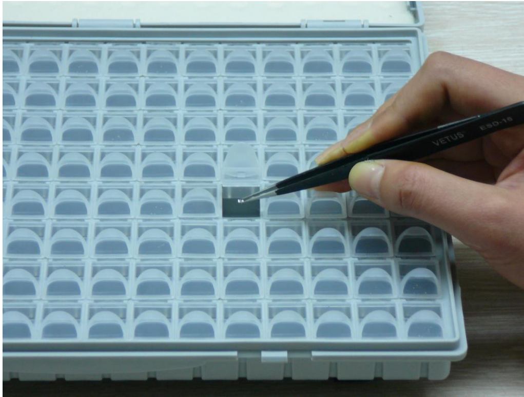
Figure 12. Storing or Obtaining an SMT Component
