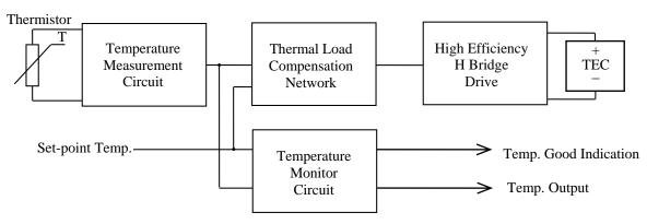
Figure 3. TEC Controller Block Diagram
