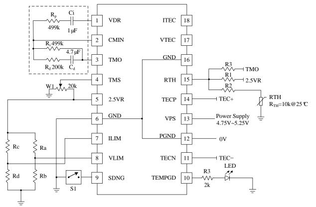
Figure 4. TEC Controller Connections
