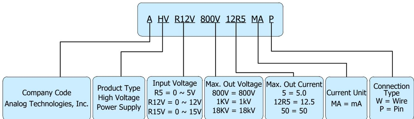
Figure 6. Naming Principle of AHVR12V800V12R5MAP
