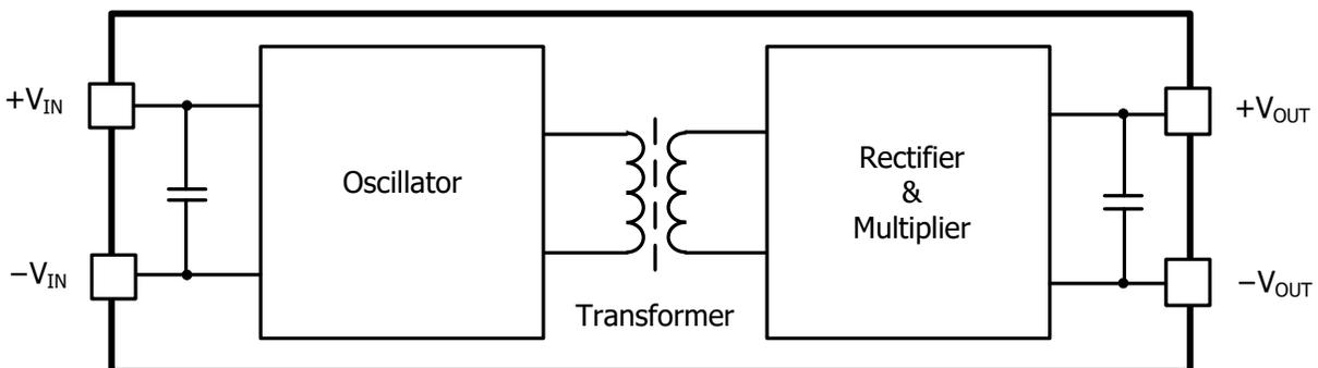
Figure 4. Block Diagram
