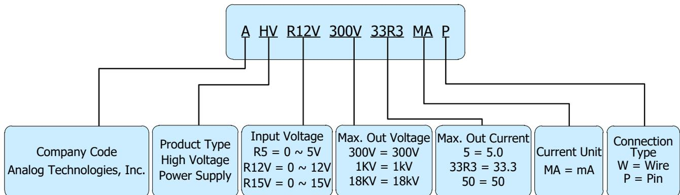
Figure 6. Naming Principle of AHVR12V300V33R3MAP
