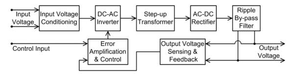
Figure 5. Block Diagram
