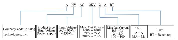
Figure 6. Naming Rules of AHVAC2KV2ABT
