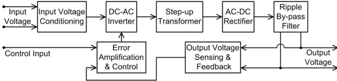
Figure 5. Block Diagram
