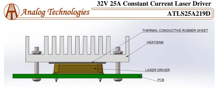
Figure 13.2 Transferring Heat with Heat Sink
