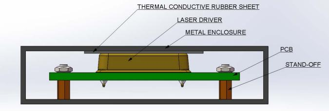
Figure 13.1 Transferring Heat with Metal Enclosure
