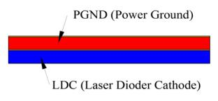
Figure 16. The Section View for the Two-Layer PCB
