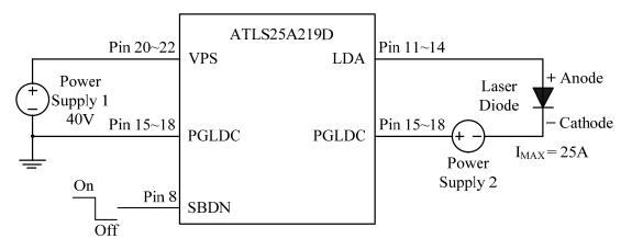
Figure 14. Driving High Voltage Laser Diodes
