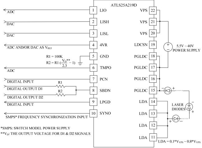
Figure 8. Micro-Controller Based Application Schematic
