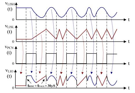
Figure 9. Digitally Controlled Analog Modulation Principle
