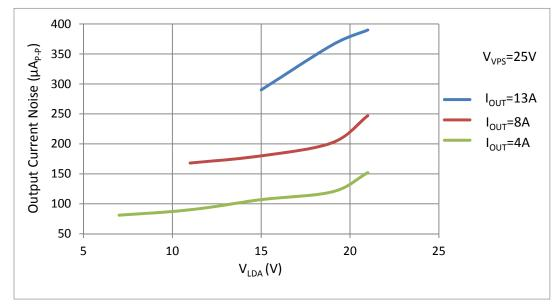
Figure 10. VLDA vs. Output Current Noise@0.1Hz~10Hz
