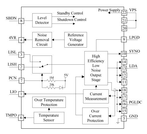
Figure 3. Internal Block Diagram of ATLS25A219D
