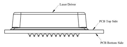
Figure 20. End View of the PCB Foot-print
