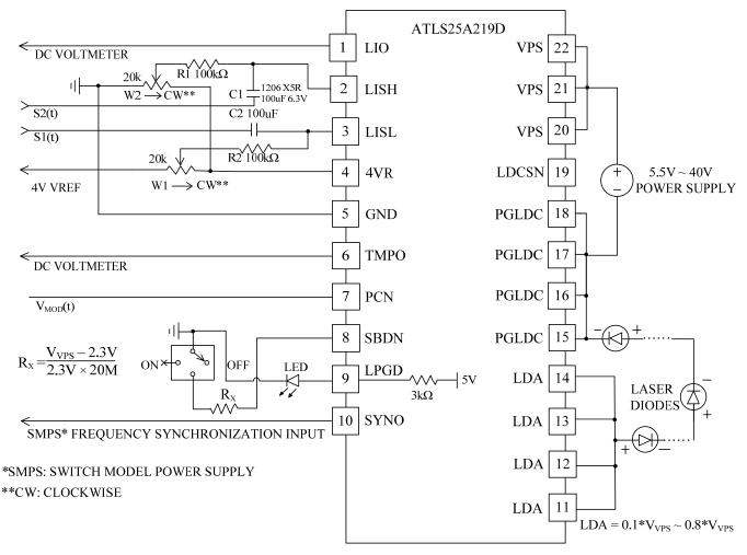
Figure 7. Stand-Alone Application Schematic
