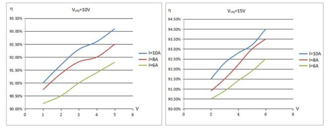
Figure 6. Efficiency of Laser Driver
