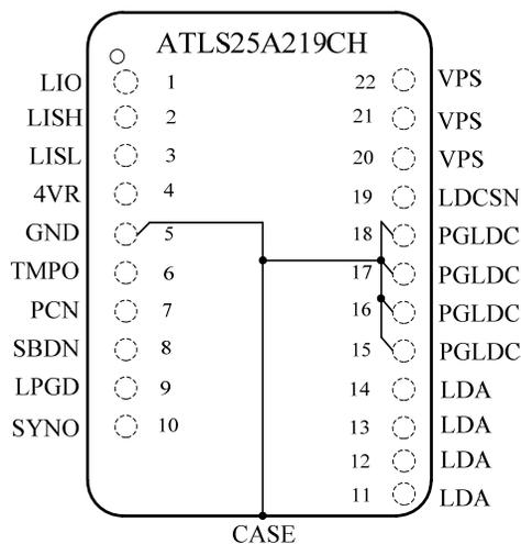
Figure 2 is the top view of the ATLS25A219CH. The pin functions and specifications are described in Table 1 below. Note that the metal case is internally connected to ground.
