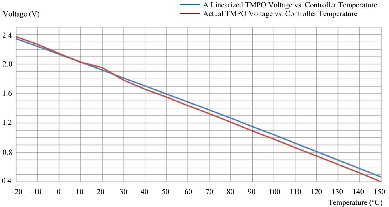
Figure 5. Controller Internal Temperature vs. TMPO Voltage
