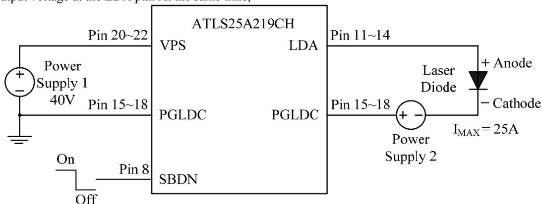
Figure 13. Driving High Voltage Laser Diodes
