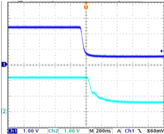
Figure 12.2. Large Signal Fall Time 220ns
