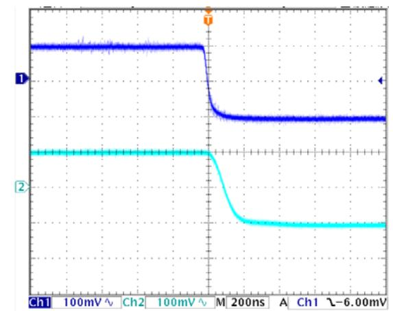
Figure 12.4. Small Signal Fall Time 200ns
