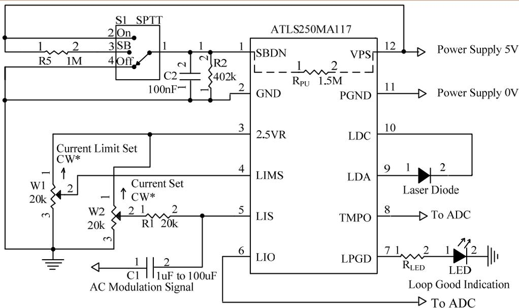
Figure 5.3. Typical AC Modulation with DC bias Schematic for ATLS250MA117
