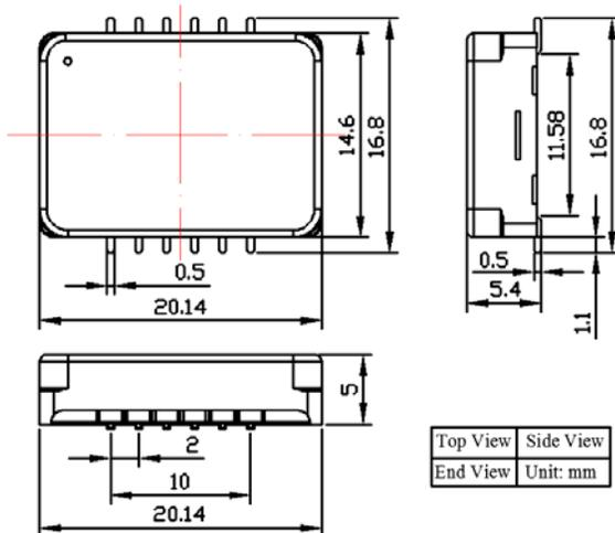
Figure 20. Dimensions of the SMT Package Controller
