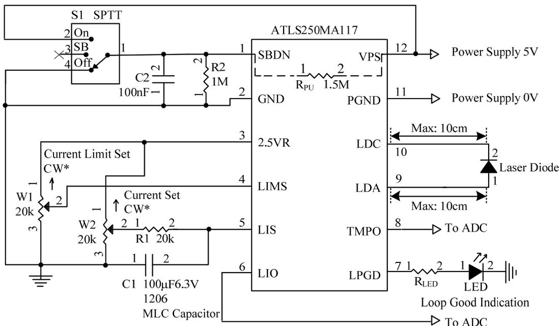
Figure 5.1. Typical Stand-alone CW Operation Schematic for ATLS250MA117
