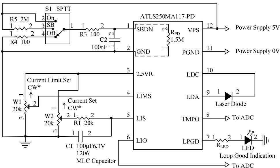
Figure 5.2. Typical Stand-alone CW Operation Schematic for ATLS250MA117-PD
