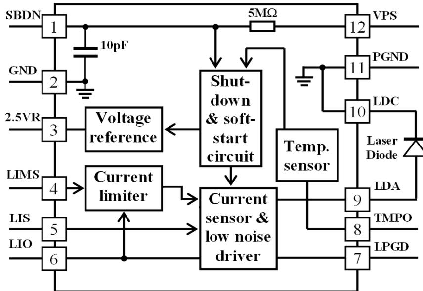
Figure 4. Block Diagram
