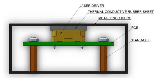
Figure 19.1 Transferring Heat with Metal Enclosure
