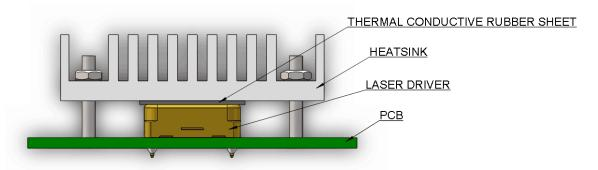
Figure 19.2 Transferring Heat with Heat Sink
