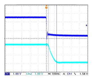
Figure 12.2. Large Signal Fall Time 100ns
