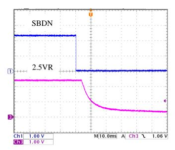
Figure 18. The fall time of SBDN vs. 2.5VR
