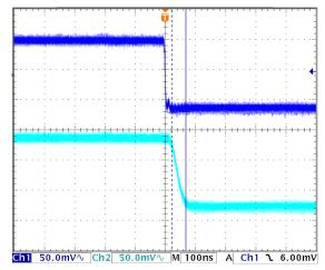
Figure 12.4. Small Signal Fall Time 46ns
