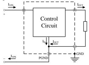
Figure 10. The Current Distributions in the Controller
