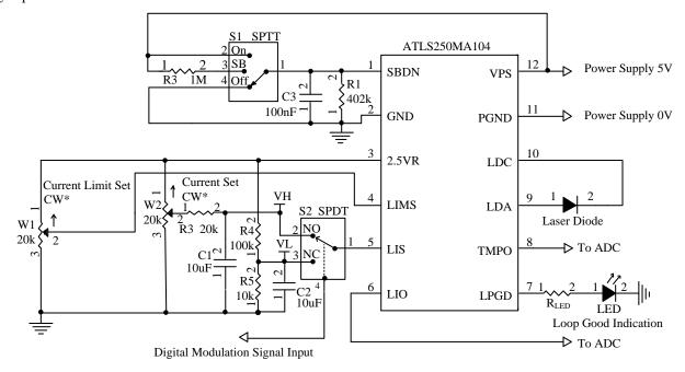
Figure 8. Low Noise Digital Modulation Circuit
