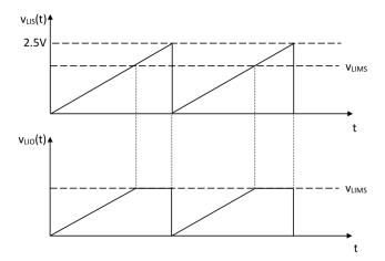
Figure 9. LIO is Controlled by LIS and Clamped by LIMS
