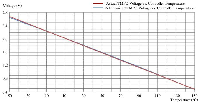
Figure 20. Controller Internal Temperature vs. TMPO Voltage
