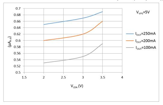
Figure 11.1. V<sub>LDA</sub> vs. Output Current Noise@0.1Hz~10Hz
