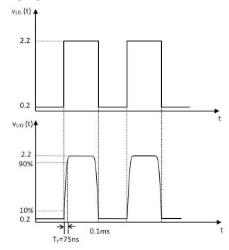
Figure 14. Large Signal Modulation
