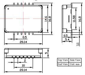
Figure 22. Dimensions of the SMT Package Controller
