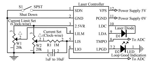
Figure 4.1. Typical Stand-alone Application Schematic for ATLS250MA103
