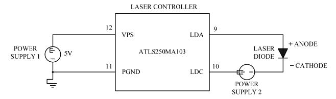
Figure 15. Driving High Voltage Laser Diodes
