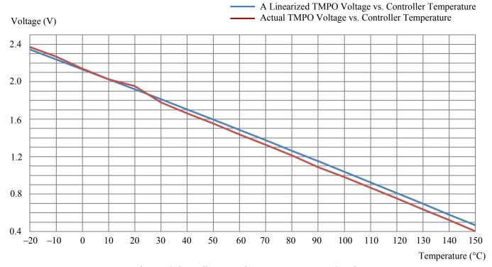
Figure 16. Controller Internal Temperature vs. TMPO Voltage
