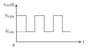
Figure 10. LIO Pin Voltage v<sub>LIO</sub> (t) Waveform
