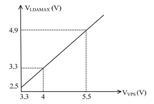
Figure 8. Power Supply Voltage V<sub>VPS</sub> vs. LDA Pin Maximum Voltage V<sub>LDAMAX</sub>
