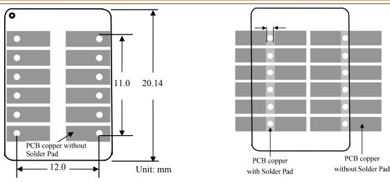
Figure 22. Top View of the Bottom Side of the Recommended PCB Foot-print
