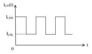
Figure 12. Laser Diode Current i<sub>LD</sub> Waveform
