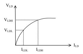
Figure 9.1. Laser Diode Current ILD vs. Laser Diode Voltage
