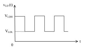
Figure 9.2. Laser Diode Voltage v<sub>LD</sub>(t) Waveform
