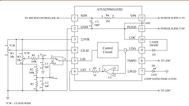
Figure 7. Low Noise Digital Modulation Circuit
