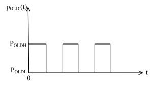
Figure 13. Laser Diode Optical Power pold Waveform
