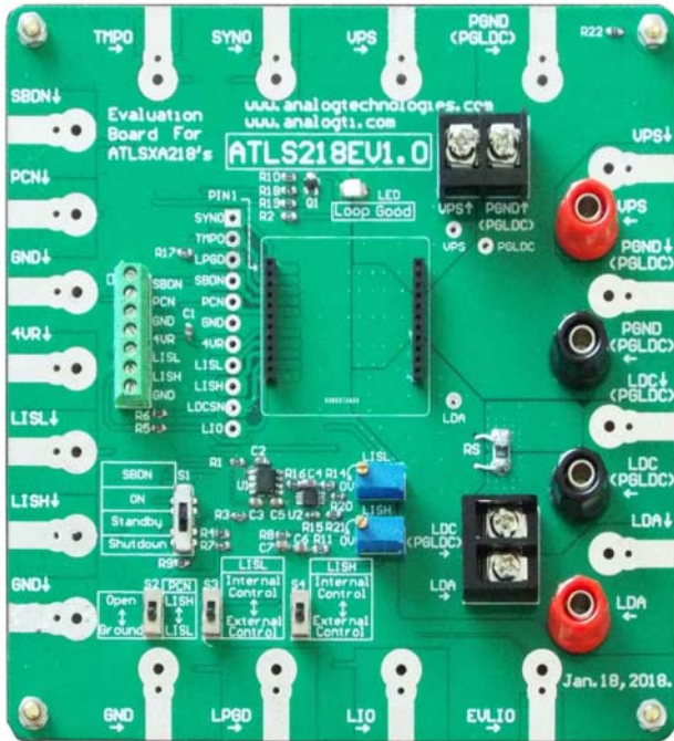
Figure 1. Physical Photo of ATLS218EV1.0
