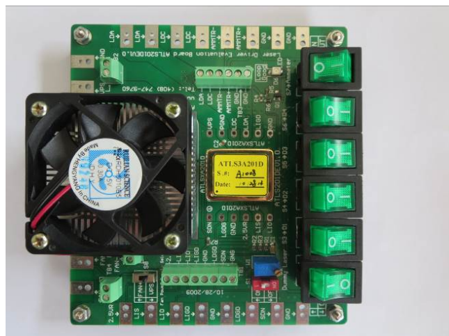
Figure 10. Side View of Actual ATLS201DEV1.0 (3)
