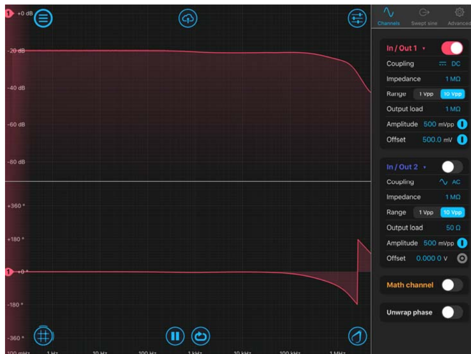
Figure 16. LIS & LIO Frequency Response Waveform
