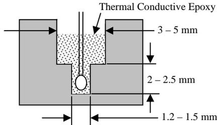
Figure 3. Section View of the 2 Stage Hole
