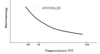
Figure 4. Resistance vs. Temperature for ATH10KL2D
