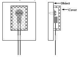
Figure 3. Using an Insulation Cover to Improve Accuracy
