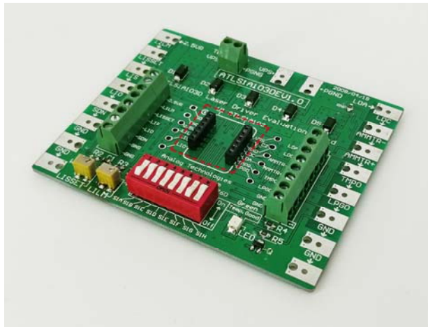
Figure 2. ATDSC2MM6P on the Laser Driver Evaluation Board
