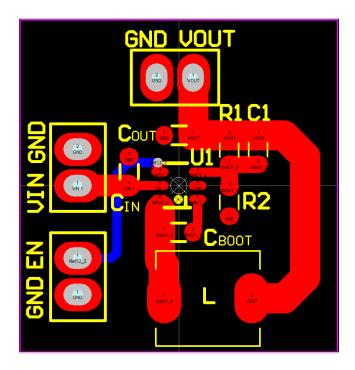
Figure 24. PCB Layout
