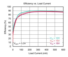
Figure 18. Efficiency vs. Load Current @ Vout=3.3V
