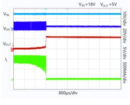
Figure 12. Short-Circuit Recovery
