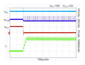
Figure 11. Short-Circuit Entry
