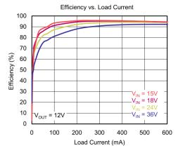
Figure 16. Efficiency vs. Load Current @ Vout=12V
