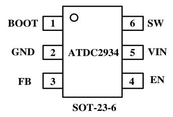
Figure 3. Pin Configuration
