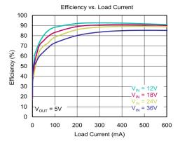
Figure 17. Efficiency vs. Load Current @ Vout=5V
