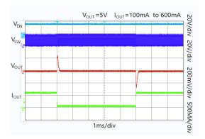
Figure 15. Load Transient Response
