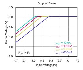
Figure 21. Dropout Curve
