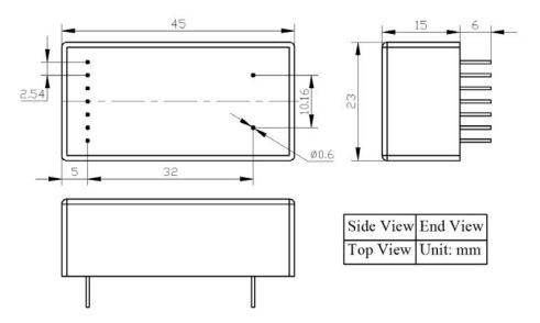
Figure 7. Dimensions for AM01HV12VP3KVR5MAP
