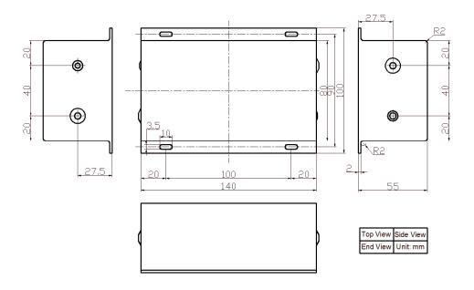
Figure 12. Dimensions for ALSHV24V6600V10MAW
