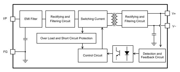
Figure 2. Power Supply Function Block Diagram
