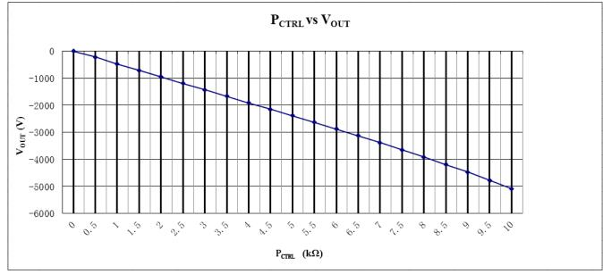
High voltage power supply testing data (Test condition: the load is  $1M\Omega$ )
