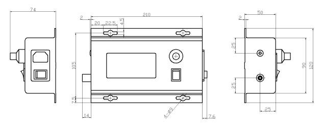
Figure 9. Dimensions for AHVACN5KV5MABT
