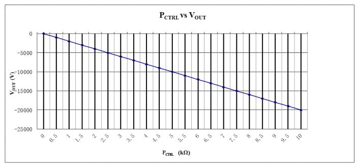
Figure 6. P<sub>CTRL</sub> vs. V<sub>OUT</sub>
