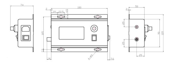
Figure 9. Dimensions for AHVACN15KV1MABT
