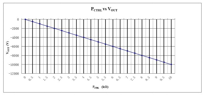
High voltage power supply testing data (Test condition: the load is 20 M $\Omega$ )
