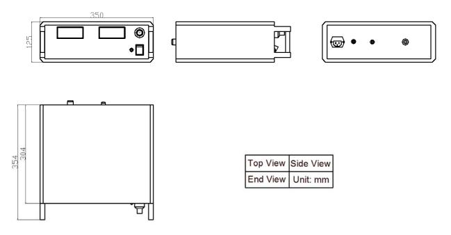
Figure 7. Dimensions for AHVACN10KV10MABT
