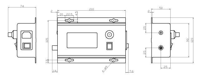
Figure 9. Dimensions for AHVACN5KV5MABT
