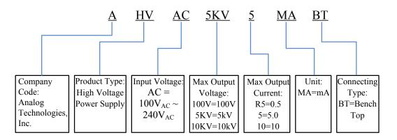
Figure 7. Naming Rules of AHVAC5KV5MABT
