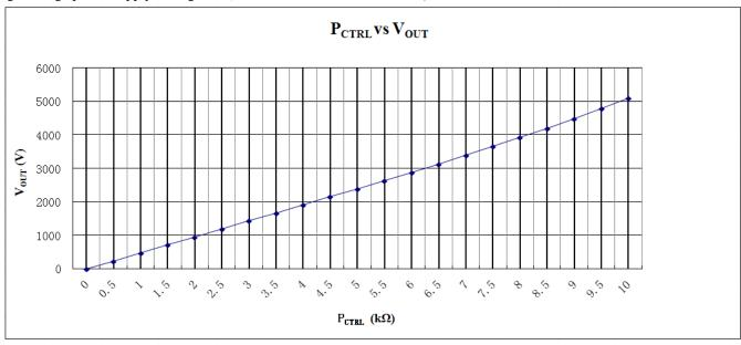
Figure 6. P<sub>CTRL</sub> vs. V<sub>OUT</sub>
