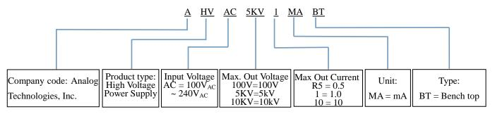
Figure 7. Naming Rules of AHVAC5KV1MABT
