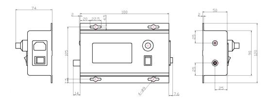
Figure 9. Dimensions for AHVAC5KV1MABT
