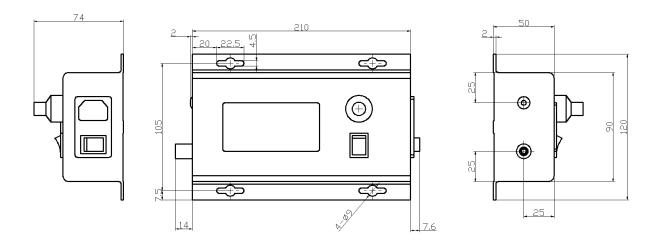
Figure 9. Dimensions for AHVAC20KVR5MABT
