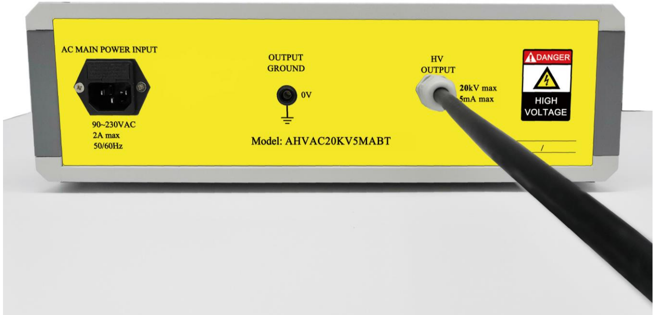
Figure 6. Leads of AHVAC20KV5MABT
