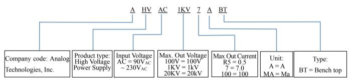
Figure 6. Naming Rules of AHVAC1KV7ABT
