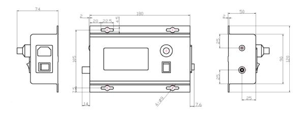
Figure 9. Dimensions for AHVAC10KVR5MABT
