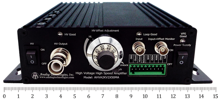
Figure 1. The Physical Photo of AHVA2KV2X50MA
