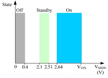
Figure 3. V<sub>SBDN</sub> vs. Amplifier States
