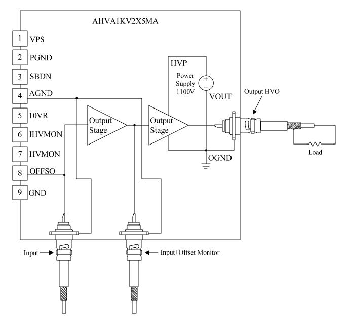
Figure 4. Schematic for Driving the Load
