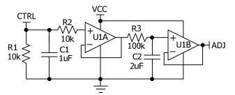
Figure 5. The Equivalent Circuit for CTRL Port
