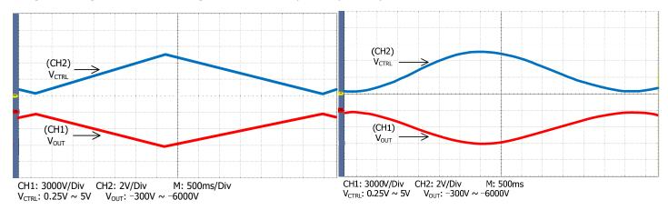
Figure 8. Input vs. Output Waveforms for Triangle Wave Control
