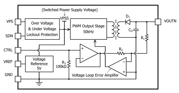
VOUTN =  $-N \times V_{CTRL}$ , where N is the amplification factor: N =  $R_1/R_2$ .
