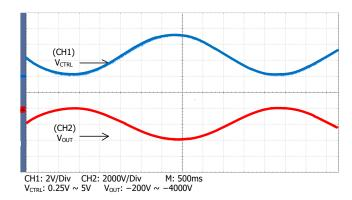
Figure 9. Input vs. Sine Wave Modulation
