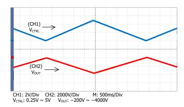
Figure 8. Triangle Wave Modulation
