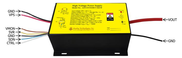
Figure 2. The Connecting Lead Wires of AHV24VN40KV1MAW
