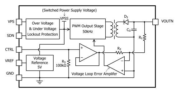
VOUTN =  $-N \times V_{CTRL}$ , where N is the amplification factor: N =  $R_1/R_2$ . High Voltage Power Supply Function Block Diagram
