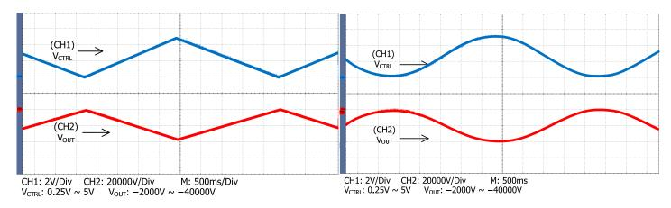
Figure 8. Triangle Wave Modulation
