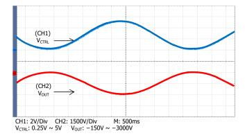
Figure 9. Sine Wave Modulation
