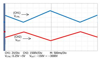
Figure 8. Triangle Wave Modulation
