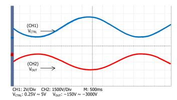
Figure 9. Sine Wave Modulation
