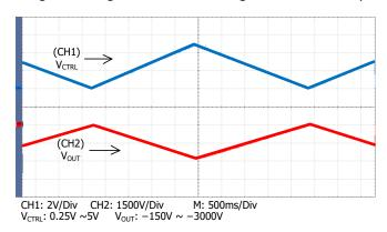
Figure 8. Triangle Wave Modulation
